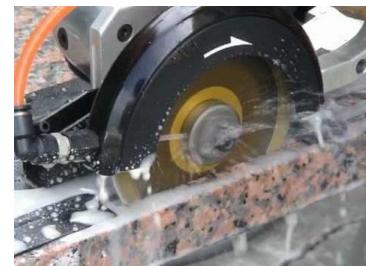
Figure 2 Wet cutting granite
